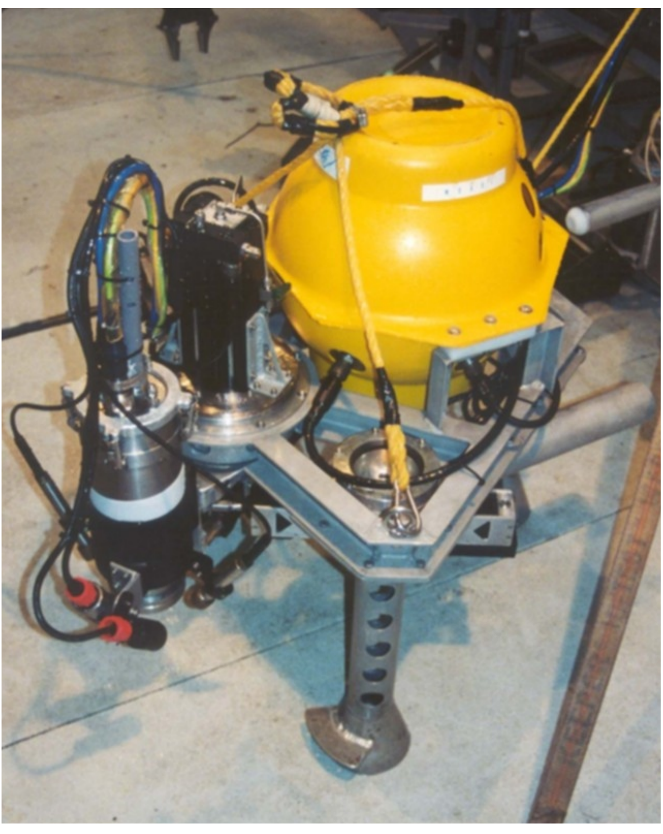
The Precision Underwater Positioner (PUP - above) was used to position the DORISS probe head.
