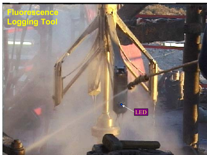
Figure 9 shows a photograph of the Fluorescence Logging Tool prototype [24]. This prototype used blue and red LED's to excite fluorescence along the borehole wall.
