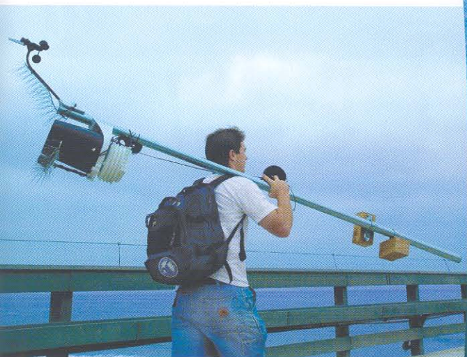
ROADNet technician Steve Foley carries a meteorological station assembled on an aluminum pole out to the end of Scripps Pier where he and technician Todd Hansen mount it on the roof of the pier shack.
