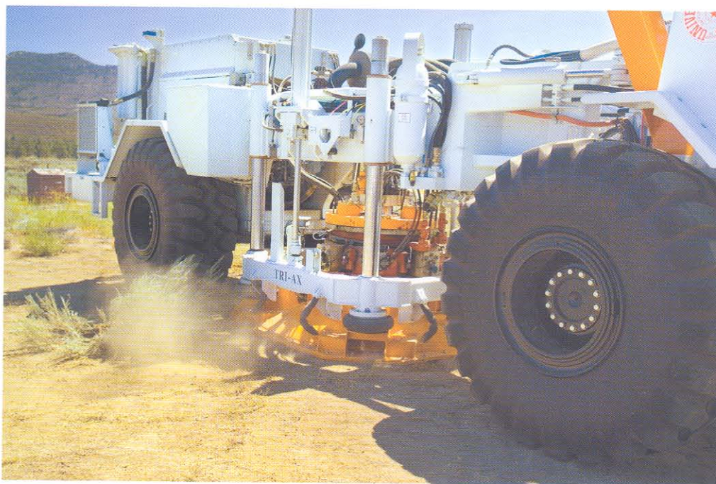
Opposite page, Frank Vernon and T-Rex, a ground-shaking truck, at the Network for Earthquake Engineering Simulation field station in Garner Valley. Left, Dust rises up as T-Rex shakes the ground with 65,000 pounds of force to simulate an earthquake. Below, T-Rex and an instrument van are operated by the University of Texas at Austin.
