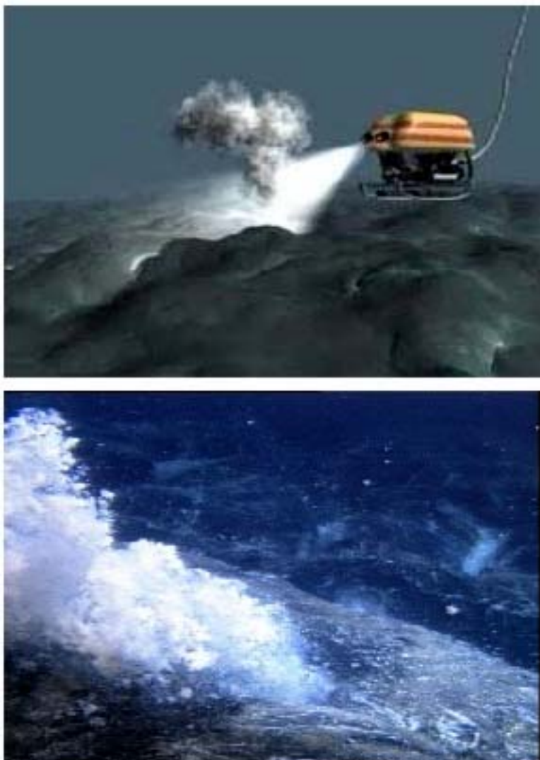
Figure 6a & 6b. Remotely operated vehicles (ROVs) may serve as important tools for sampling at cabled observatory sites. Copious outpourings of white flocculent material called “snowblowers” are a distinctive form of low-temperature hydrothermal vent. Unlike high-temperature black smokers, where the suspended material in the “smoke” is tiny mineral particles, the “snow” is biological in origin. It is a byproduct of a microbial bloom in the subsurface hydrothermal system. Observatory studies may help determine how volcanic eruptions invigorate the subseafloor biosphere and create these blooms. The top image is a virtual image and the bottom image is a photo from Axial Caldera.
