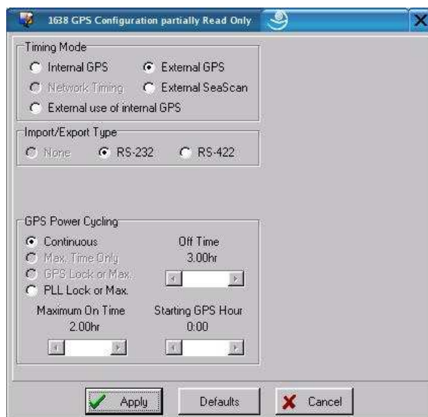
Figure 5: Q330 configured as a time client.
