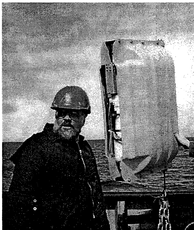
Fig. 3, The "Seahorse" Profiler showing the opening at the back where sensors are mounted.
