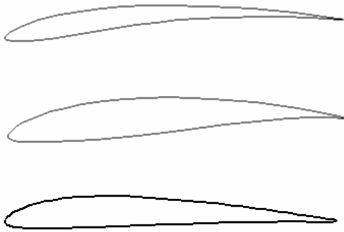
Figure 4. Low Reynolds number airfoils [3]. From top to bottom E214, GM15 and WASP
