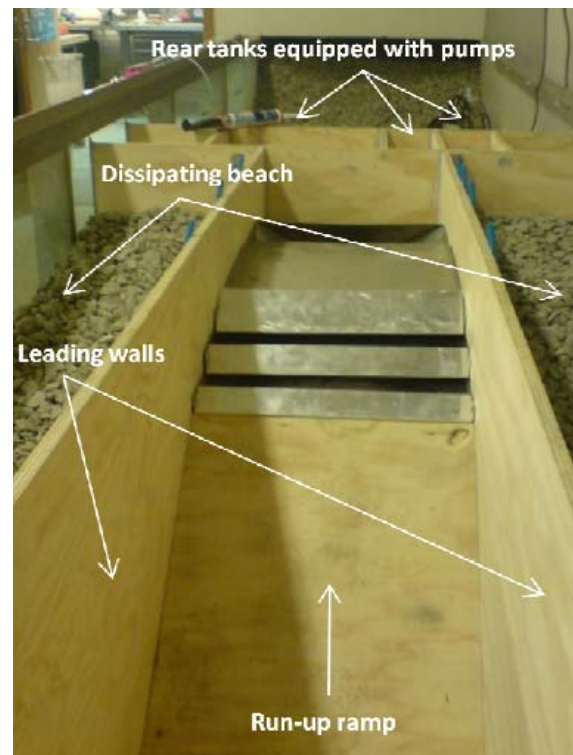
Figure 1: Frontal view of the SSG device with 3 reservoirs.
