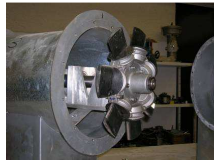
Figure 3 .- The small scale model of the Wells turbine off the air tube.
