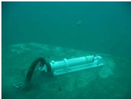
Figure 6: Current profiler installed.
