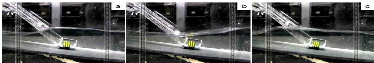
Figure 6 Frameshots of incoming wave exerting force on the pump at non resonant conditions. (a) Incoming Wave and measurement of wave height on the slope; (b) maximum wave height achieved and (c) maximum lift height.
