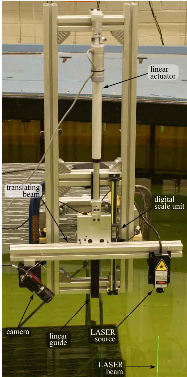
Figure 3: Optical wave gauge and calibration rig assembly set up in the Edinburgh curved tank. One can see the line of scattered light created by the LASER beam below the water surface.
