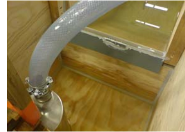
Figure 4: Detailed view of overtopping detection system and pump inside reservoir.
