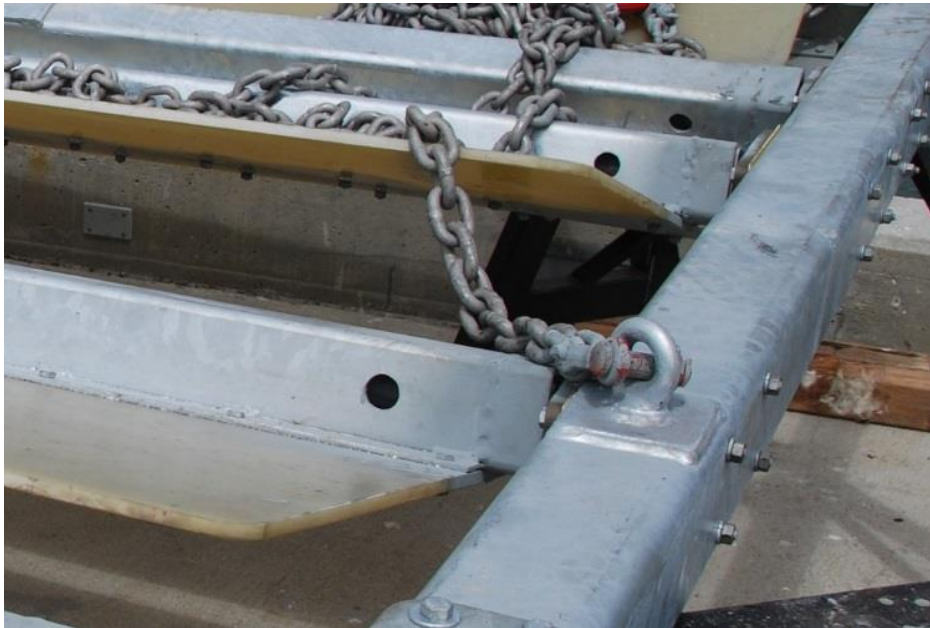
Pad eye, clevis connector and chain on the compliant plate.
