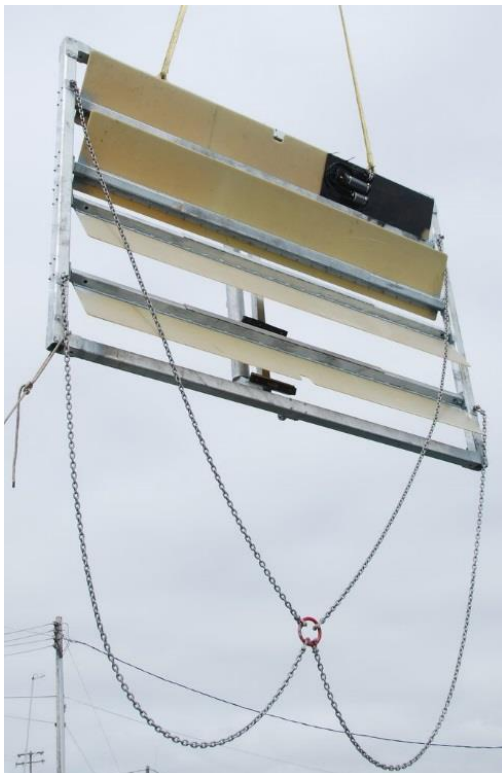
Chain bridle attached to the compliant plate.
