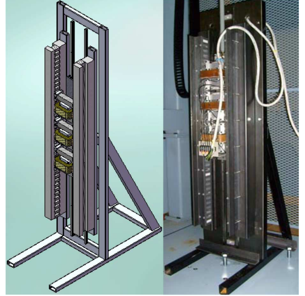
Fig. 4. Vernier hybrid generator PTO model and hardware.
