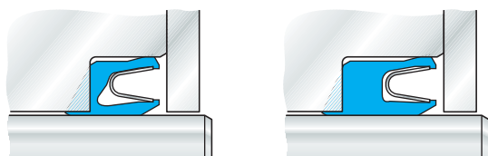
Figure 5.3 – Extended heel minimizes extrusion damage
