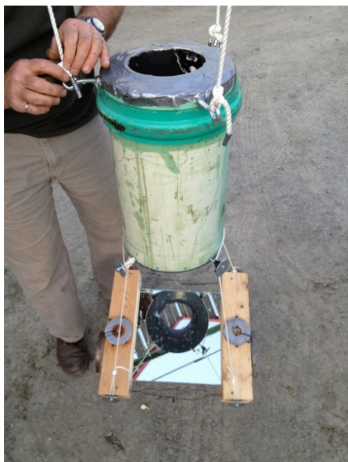
Figure 4.2.2 Set-up for the laser fluorescence installation. An insulated PVC tube with a mirror beneath was used to keep a clear optical path from above the ice (left). Laser system viewed from behind (below).
