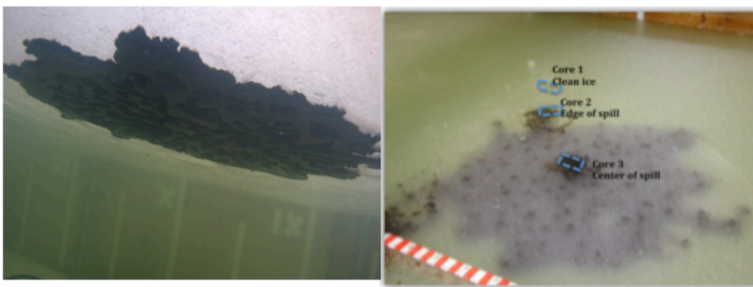
Figure 4.3.6 The oil spill under nilas viewed from below showing an undulating topography (left). The spill could be seen from the surface due to the thin ice, although little oil percolated through. A pock-marked appearance resulted from oil percolating part way through brine drainage features. The location of cores taken after the experiment is indicated. Note the oil on the surface is due to spillage during deployment or taking of cores.
