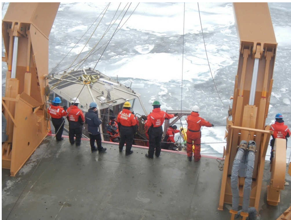
Figure 3.2.3. Recovery of the AUV by small boat in 100% ice cover.
