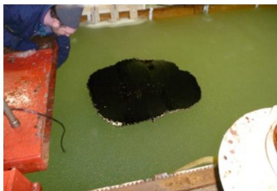
Figure 4.3.4 Oil pushed its way through the frazil layer and spread over the surface.
