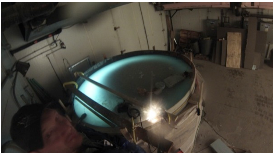
Figure 4.2.1 The test tank viewed from above, with illumination provided from below. Note the dark area in the center where the oil was deployed beneath the ice.
