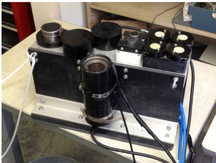
Figure 4.7 The sonar transducers mounted at the bottom of the test tank. From left to right: Marine electronics 1.1 MHz profiler, two 160 kHz Airmar transducers for the broadband system, two 500 kHz Airmar transducers for the broadband system, and four Aquascap transducers (there 1 MHz (two connected) and one 5 MHz). A Prosilica low-light camera is mounted in an underwater housing on the side of the instrument platform.
