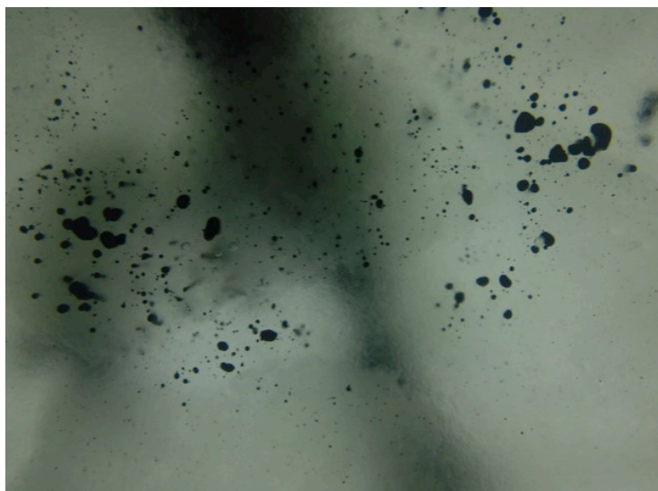
Figure 6.1.5 Upward looking photos of the spill pancake ice at HSV A immediately after the spill. This is the only location where significant droplets remained under the pancakes. Most of the oil was forced between the pancakes, where the color contrast may be difficult to distinguish from variability in the ice thickness or overlying snow cover. Photo taken in ambient light.
