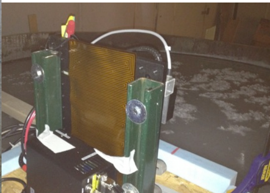
Figure 4.2.2 Set-up for the laser fluorescence installation. An insulated PVC tube with a mirror beneath was used to keep a clear optical path from above the ice (left). Laser system viewed from behind (below).
