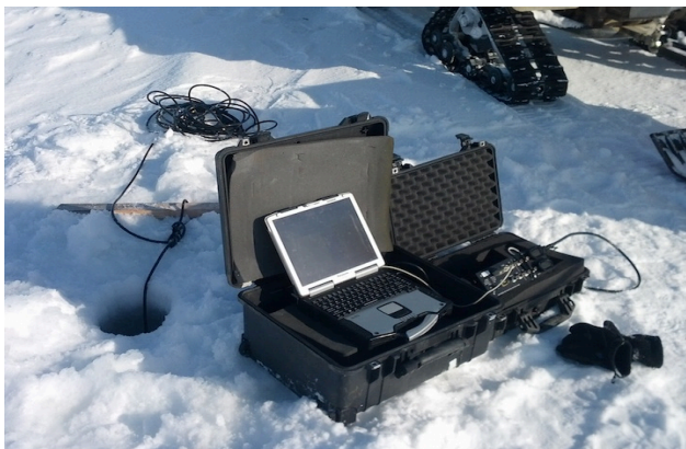
Figure 3.4.1 Laptop (left) and acoustic modem (right) with ice hole for transducer in background.
