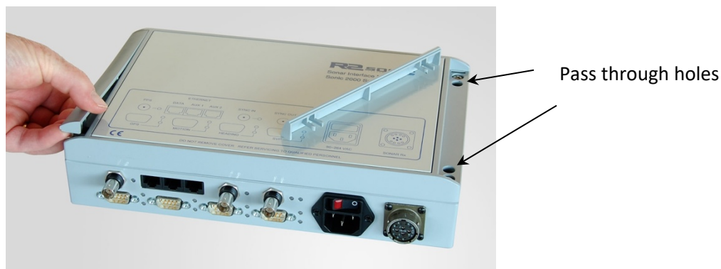
Figure 12: Removal of trim to expose securing holes
