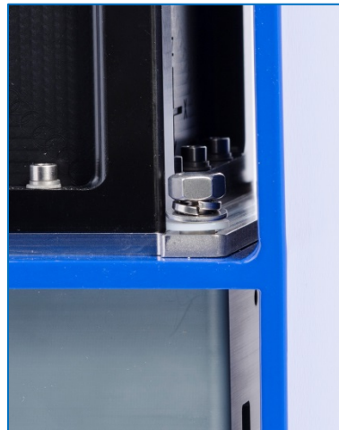
Figure 120: Detail of securing IMU and Sonic 2020
