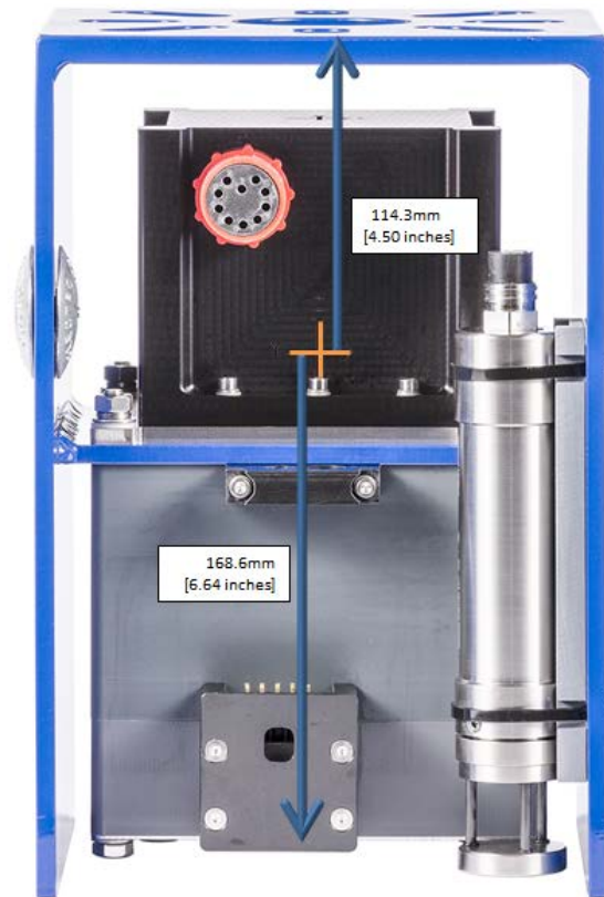
Figure 137: 2020-INS Vertical Offsets
