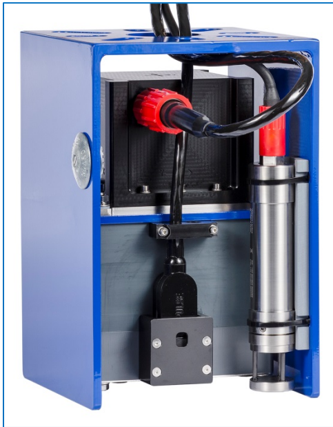
Figure 121: Aft detail of the IMU cable connection
