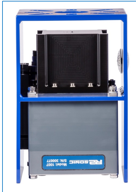
Figure 119: IMU mounted within the Sonic 2020 mounting frame
