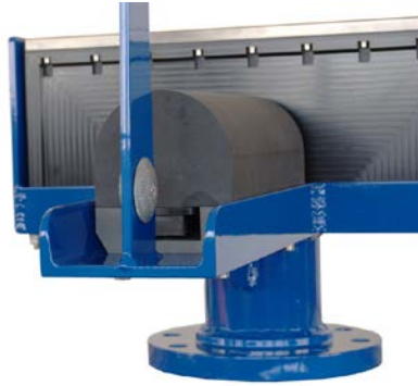
Figure 28: View of the mounted Projector; NB. The connector is facing protective fin
