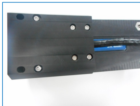
Figure 21: Projector cable clamp in place
