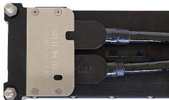
Figure 11: Seated connectors (Sonic 2024 on the left and Sonic 2022 on the right)
