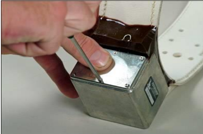
Fig. 1 Removing screws from TGW-4601
