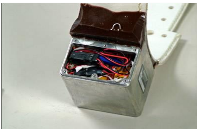
Fig. 4 All packs installed, Power leads folded down
