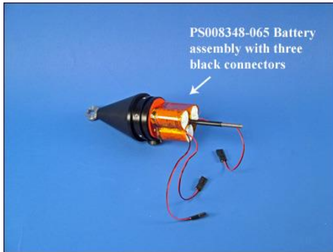
Fig. 5 Nose cone and battery assembly with black connectors installed
