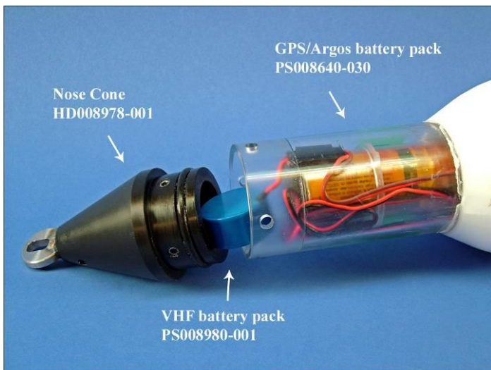
Fig. 6 VHF battery pack connected to matching connector.
