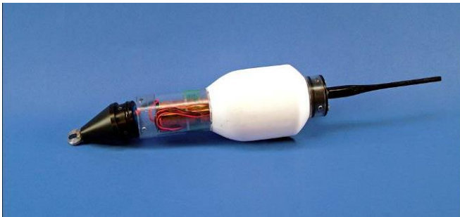
Fig. 1 Screws removed and nose cone disengaged from TMT-464-2 and TMT-464-3
