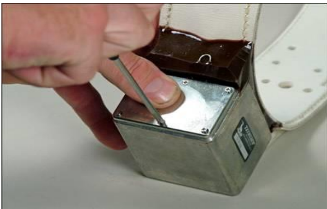
Fig. 6 Tightening screws, middle first
