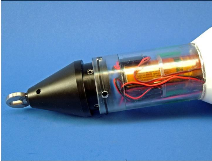
Fig. 9 VHF battery pack in nose cone cavity with nose cone ready to be inserted in housing.
