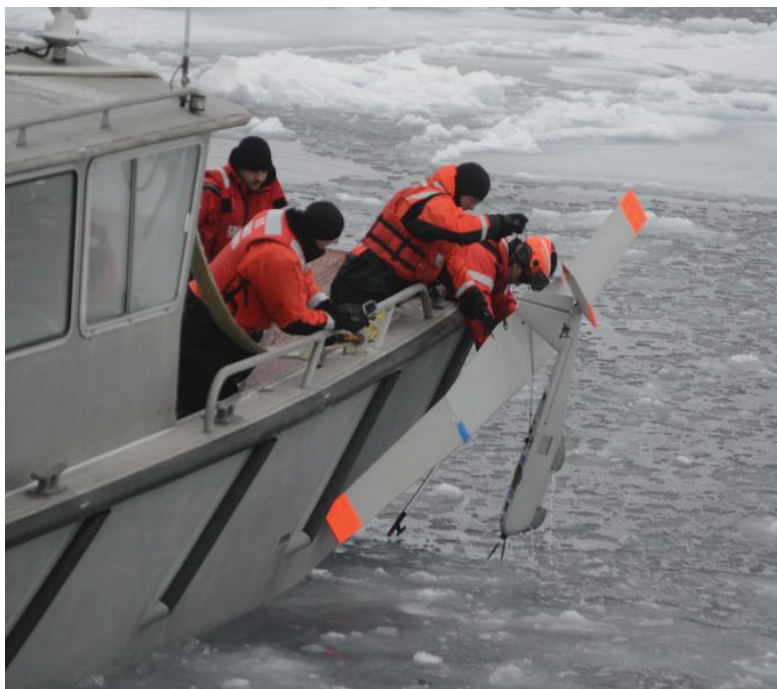
FIGURE 4-6 U.S. Coast Guard crew testing a Puma AE UAS to identify the extent of simulated spilled oil in the Beaufort Sea in 2013.
