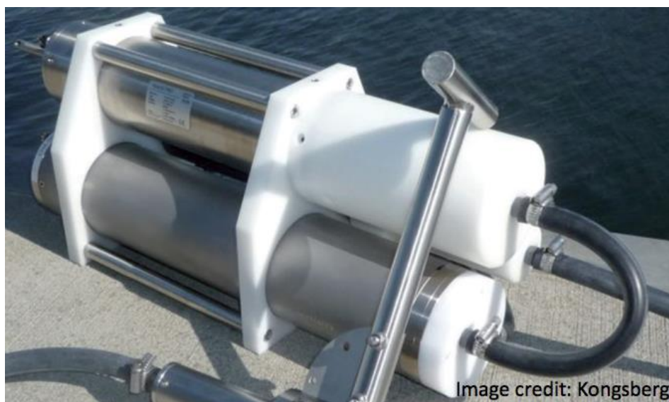
Figure 13: Kongsberg/Hydroid CONTROS MELDS sensor suite.
