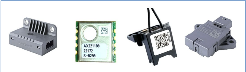
Figure 5 - Advanced Battery Sensors for Smoke, H2, Water, and Pressure
