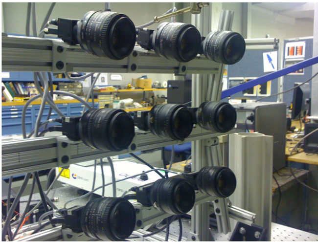
Figure 13. Photograph of the camera array. Nine cameras are mounted with 50 mm lenses on an extruded aluminum frame. Only eight cameras are used in the study.
