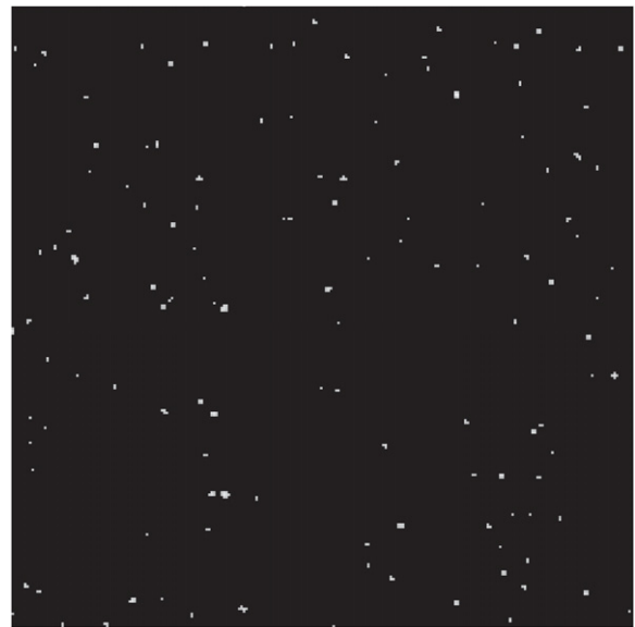
Figure 5. Zoomed view ( 250 \times 250 pixels) of the thresholded refocused image from figure 3(b) revealing the particles and removing the background noise.
