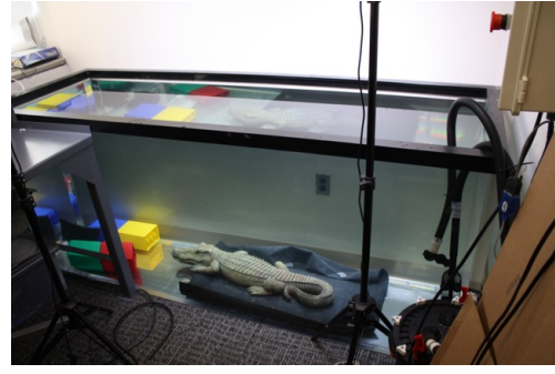
Fig. 4. Laboratory water tank setup and target object for reconstruction. Lighting and water clarity can be tightly controlled enabling us to test the limits of the proposed approach.
