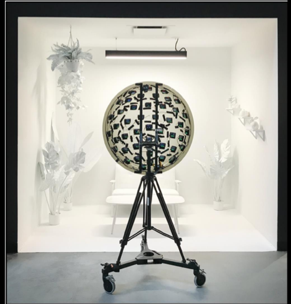
Fig. 3. Our camera array is built using a low-cost, semi-transparent acrylic dome. (a) Cameras are placed at vertices of an icosahedral tiling of a 0.92 m diameter hemisphere. This yields an average inter-camera spacing of 18 cm. (b) The plastic dome acts as a natural viewfinder, making it easy to compose a shot by looking through the surface of the camera rig.
