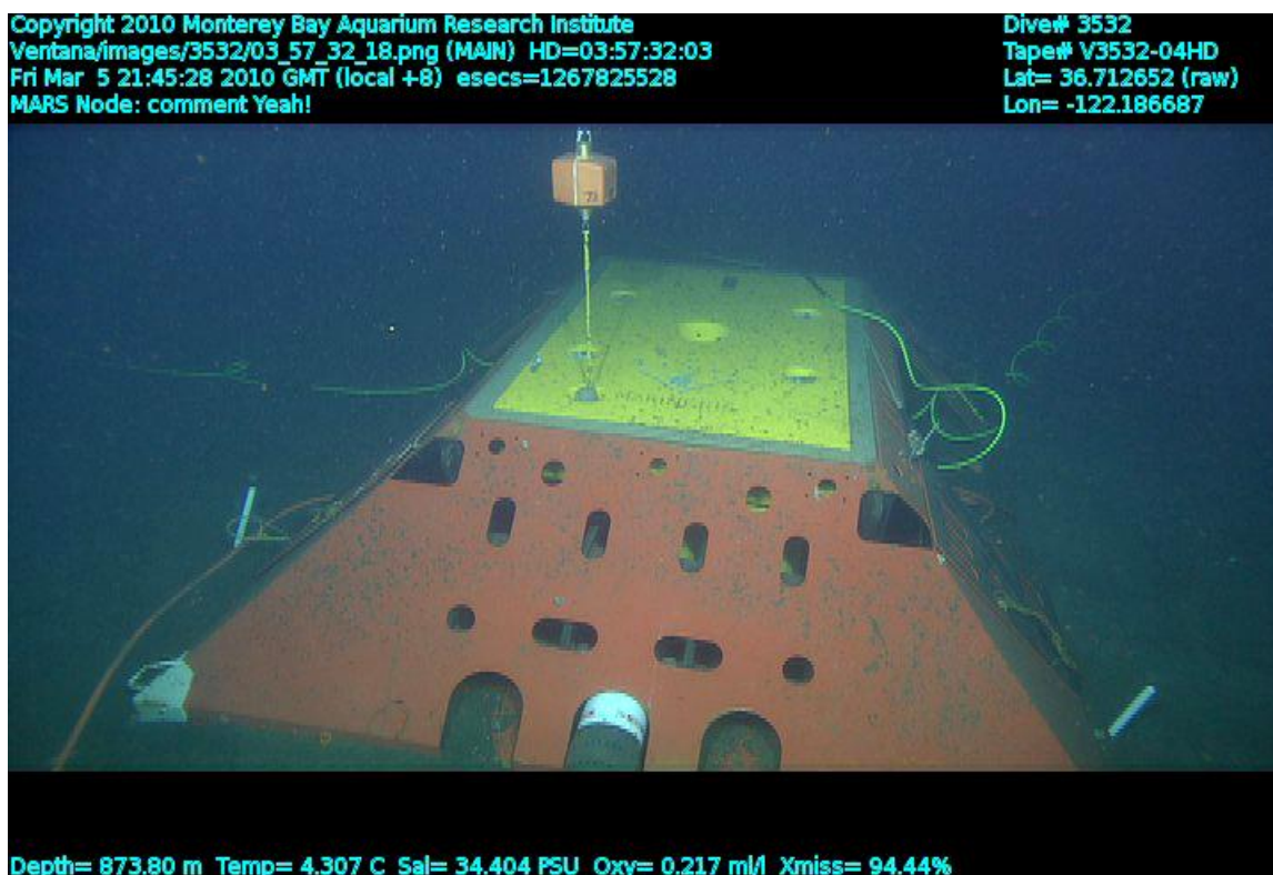
Figure 7. The MARS node with cables attached to four working science instruments.
