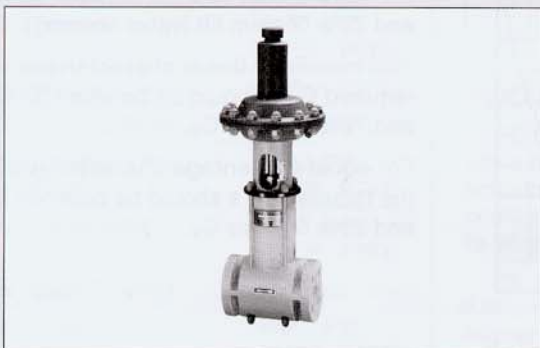
EC Series Valve has direct acting actuator accepting 3-15 psi signal without positioner.
