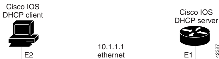
Figure 15 Topology Showing DHCP Client with Ethernet Interface
