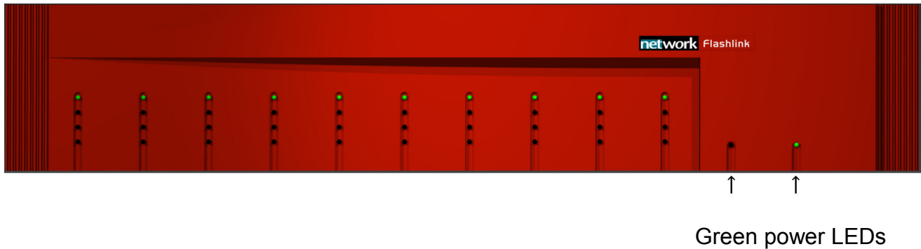
Figure 3 The front of FR-2RU-10-2-F, showing the power LEDs.
