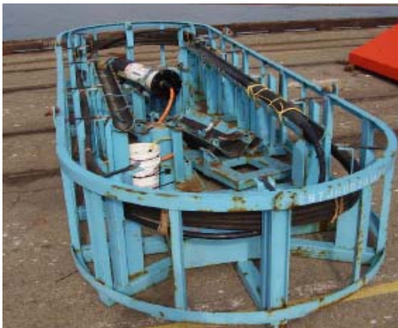
Fig. 1 – CTA, Tail & Transportation Box
