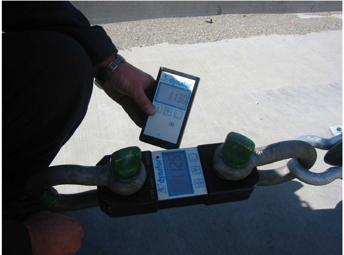
Load applied to cable 1.130 Tonnes
