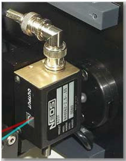
A white-light laser beam enters the PCAOM crystal from the right, while a radio-frequency signal is injected from the top. The RF signal sets up a diffraction pattern which acts as a prism.
