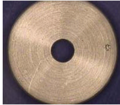
Polarizers over ring light source and lens
