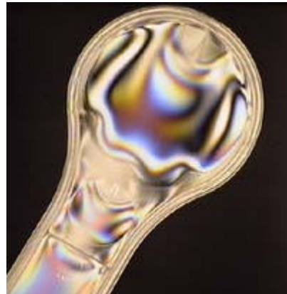
Polarizers before and after transparent object
