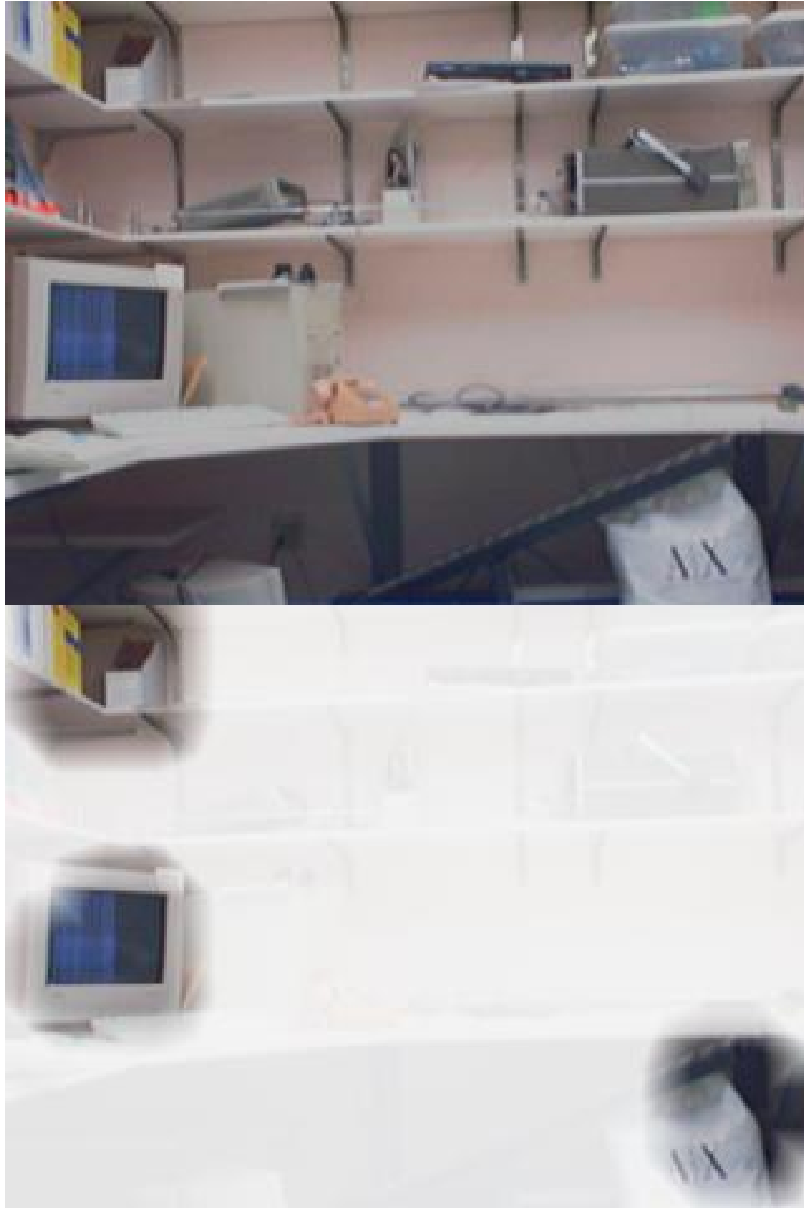
Figure 4: An example from the supplementary video provided. In the upper part the original 320x240 frame as recorded by the camera of the robot is shown and in the lower part the 3 most salient patches as used for learning and recognition are shown. We provide a MPEG1 encoded version of the video in the supplement. Additional versions (MPEG4, WMV) are provided on http://www.klab.caltech.edu/~urut/cvpr04 .
