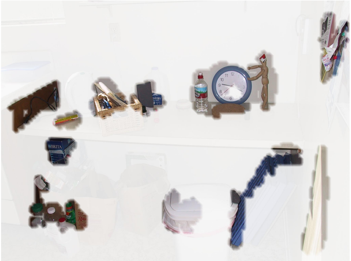
Figure 3: The 15 most salient patches of one indoor image shown merged as a cumulative image. The background (not selected parts of image) is shown slightly to provide context.
