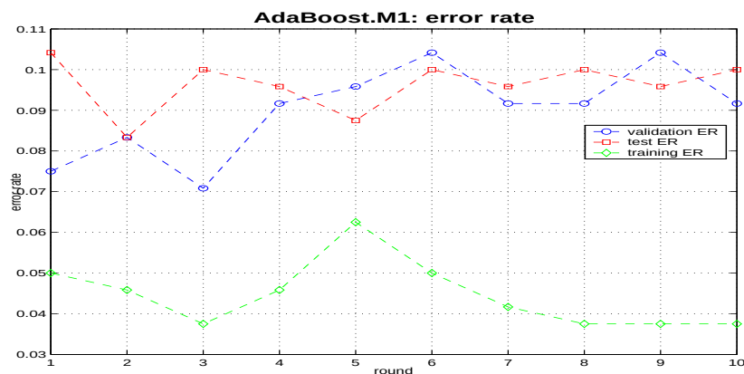
Figure 7.13: AdaBoost.M1: test, validation and training error rate as a function of the number of rounds. Training done on 480 images, each test on 20 images (randomly chosen).
