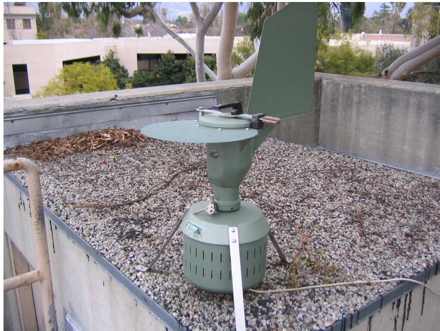
Figure 2.1: Burkard volumetric spore trap is used to collect airborne pollen grains and fungi.
