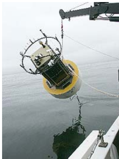
The new CIMT mooring being lowered into the calm early morning sea. Photo Kent Headley (c) 2004 MBARI
