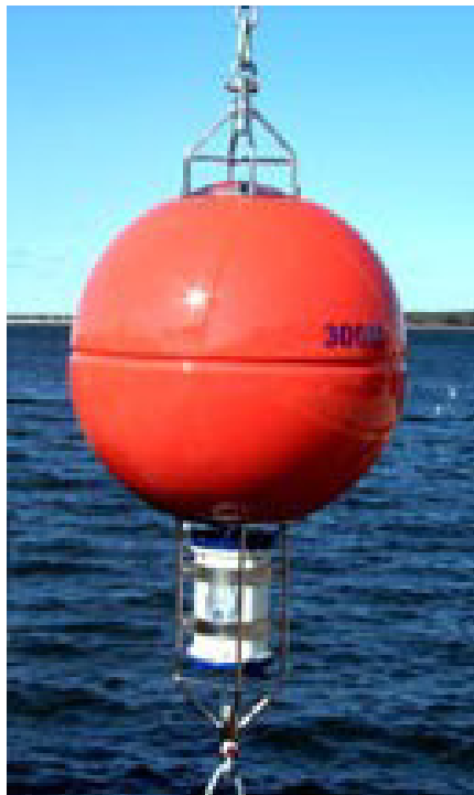
Figure 6. Buoy Mount with External Battery
