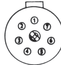
FRONT VIEW XSL-7-CCP-PBOF (7# 16 AWG)
