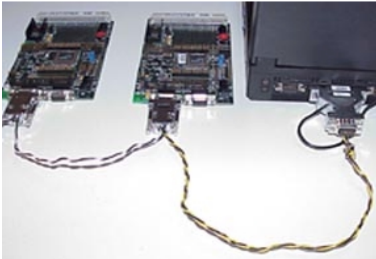
Figure 3: Three-Node CAN Network with PCAN-Dongle and two phyCORE-591 RDK
