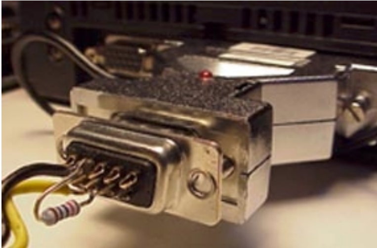
Figure 1: View of the PCAN-Dongle with DB-9 CAN Connector and 120 Ohm Termination Resistor
