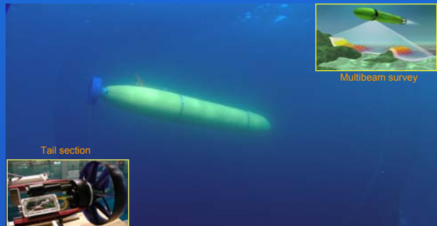
Figure 1: Dorado AUV – This is an actual frame grab from the ROV Ventana which shows the Dorado AUV autonomously diving.
