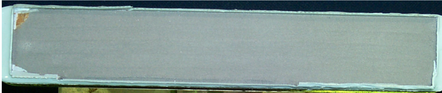
Mg Anode after 50 hours
