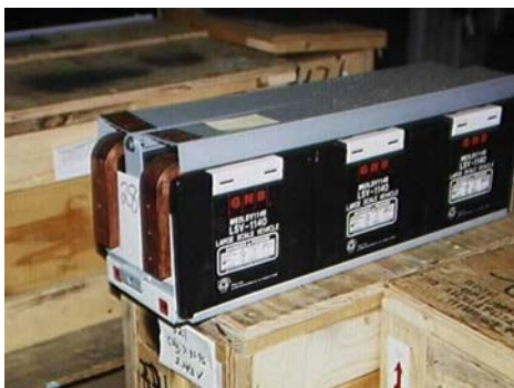
Fig. 5. The LSV-153 was replaced by a VRLA package based on a COTS battery design.
