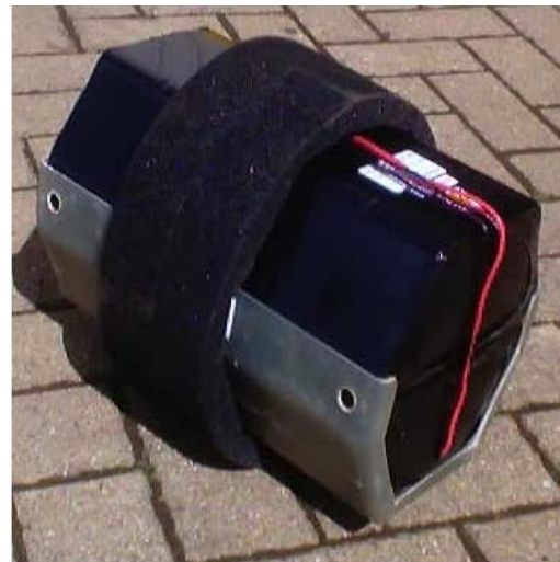
Fig. 2 Single battery pack in GFRP tray with a section of foam insulation around it
