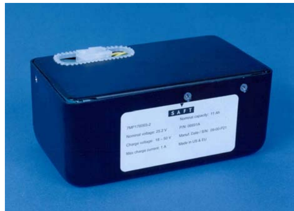
Figure 3: REMUS/SAHRV lithium ion battery brick
