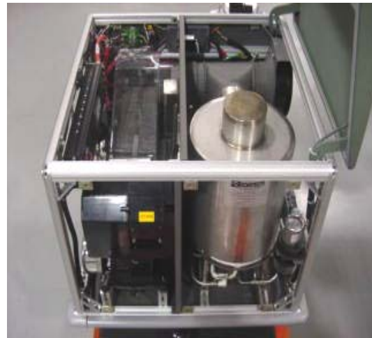
Figure 1. A 1 kW PEMFC system showing the fuel processor at the lower right and the fuel cell stack at the left.
