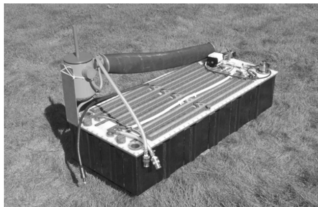
Fig. 4. Battery box (cell stack).
