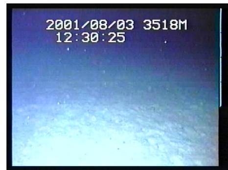
Fig.11 TV camera image transmitted by acoustic telemetry
