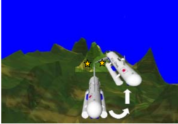
Fig. 9. The UUV changes the angle between the robot hand and the target object.
